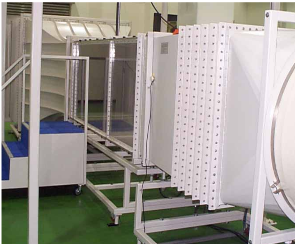
圖12 吸氣式開迴路風洞：前整流段至後整流段特寫
