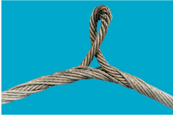
圖 112 抗旋轉鋼索內部擠出 Protrusion of inner rope of rotation-resistant rope
