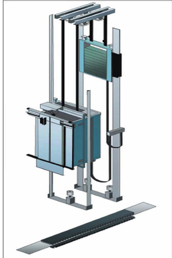
Illustration 2: A "conventional" linear motor elevator
